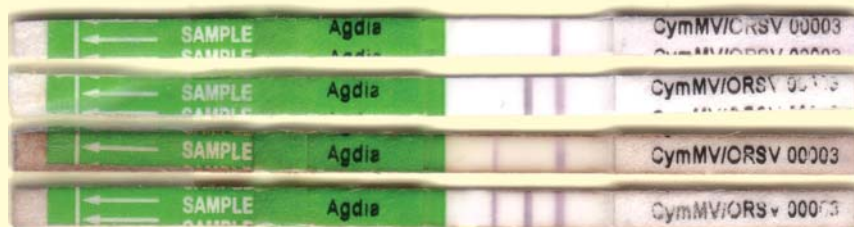
Step 5 Read the strips. A = CyMV indicator line; B = ORSV indicator line; C = control line.
